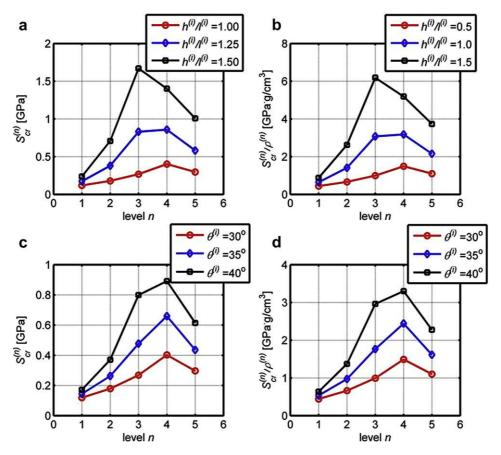
**Fig. 8.** (a) Influence of h/l on buckling strength when  $\theta = 30^{\circ}$ ; (b) Influence of h/l on strength-to-density ratio when  $\theta = 30^{\circ}$ ; (c) Influence of  $\theta$  on buckling strength when h/l = 1.0; (d) Influence of  $\theta$  on strength-to-density ratio when h/l = 1.0.
