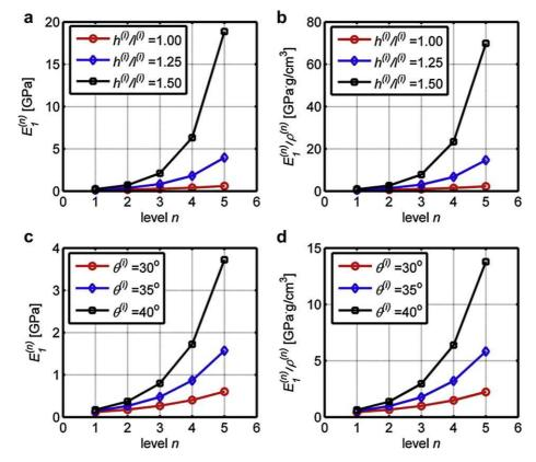
**Fig. 7.** (a) Influence of h/l on stiffness when  $\theta = 30^{\circ}$ ; (b) Influence of h/l on stiffness-to-density ratio when  $\theta = 30^{\circ}$ ; (c) Influence of  $\theta$  on stiffness when h/l = 1.0; (d) Influence of  $\theta$  on stiffness-to-density ratio when h/l = 1.0;
