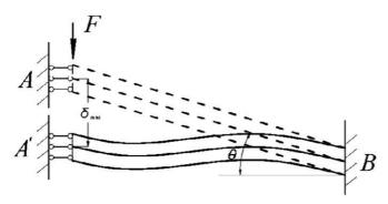
Fig. 2. An inclined orthotropic beam with one end guided and the other fixed.
