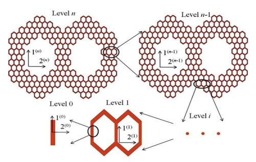
Fig. 4. Top view of the schematic of the n-level nano-honeycomb.
