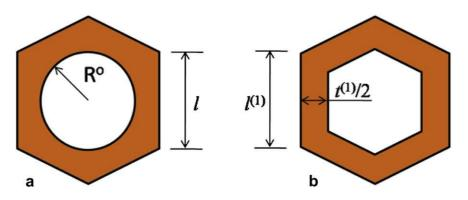
Fig. 5. (a) Unit cell of the honeycomb structure with cylindrical nano-channel; (b) Unit cell of the honeycomb structure with hexagonal nano-channel.
