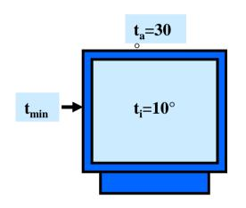
Risk of external condensation if internal temperature is lower than external temperature!
