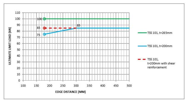
Fig. 4 b. Recommended ULS vertical shear capacity for RVK/TSS 101 in 200-265 mm slabs
