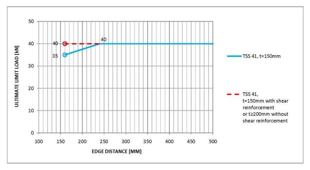
Fig. 4 a. Recommended ULS vertical shear capacity for RVK/TSS 41 in 150 mm thick slab.
