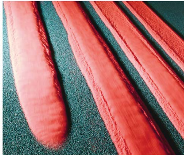
◀ FIG. 4: (left) Numerical simulation of a granular flow from a constant inflow mass flux propagating steadily downslope and spontaneously forming static levees on either side of the central flowing channel. (right) Corresponding self-channelization experiment using monodisperse red sand on a non-erodible bed (Rocha et al. 2019).
