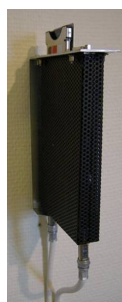
Installation on wall as a stand alone unit with single power supply (ESP-100) and a wall mount plate..
