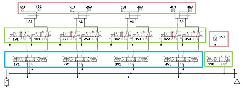
The Safety Functions can be applied to each individual actuator (A1, A2, A3 and A4); however, they can be considered a single Safety Function since they are implemented utilizing the same SRP/CS. Each Actuators Safety Function is executed at the same time.
