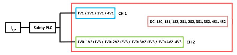
It had been identified previously that the required Category and  $PL_r$  be Category 3 PLd. The following example evaluation will determine if the identified circuit along with its components will adhere to the required Category and PL rating.
