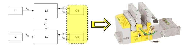
Unique components (in yellow) represent the Output Device in each channel identified above. The complete Zoned Safety Manifold integrates these required functions into and easy to render pneumatic system that allows for the required Safety adherence. See section 2 for further breakdown of the complete Zoned Safety Manifold. Complete adherence up to Category 4 requires implementation of the Input Device and Logic Element in addition to the Zoned Safety Manifold.
