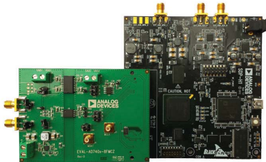
Figure 2. EVAL-AD7402-8FMCZ Evaluation Board (Left) Connected to the EVAL-SDP-CH1Z Board (Right)
