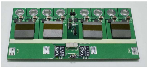
Fig. 18 Prototype of 1MHz 1kW 400V/12V LLC converter
