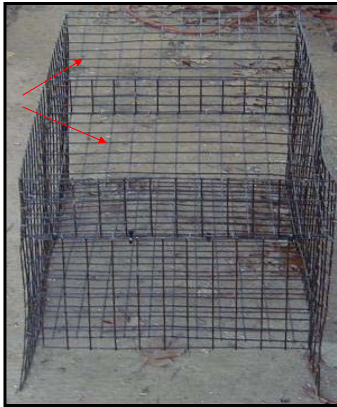
Figure 13. Funnel design with braces indicated by red arrows.
