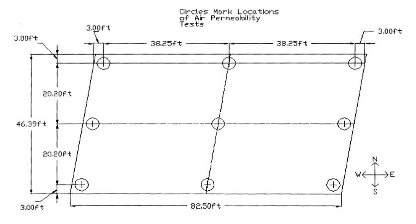
Fig. 3.38: Locations of Surface Air Flow Permeability Readings Wyckoff Road Westbound
