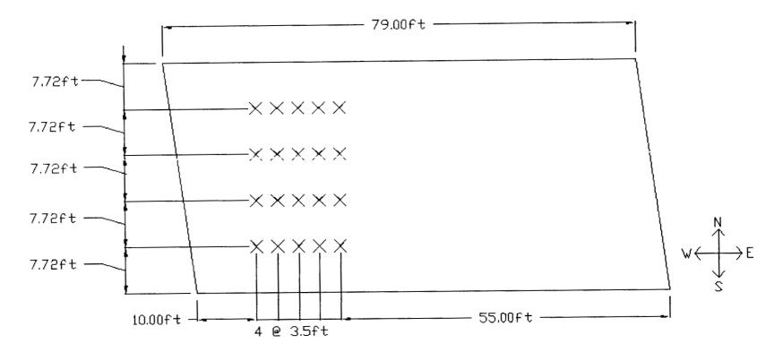
Fig. 3.12: Locations of GECOR 6 Corrosion Rate Meter Tests North Main Street Eastbound
