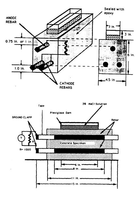
Fig. 3.10: V ew of Concrete Minideck (ASTM G 109)
