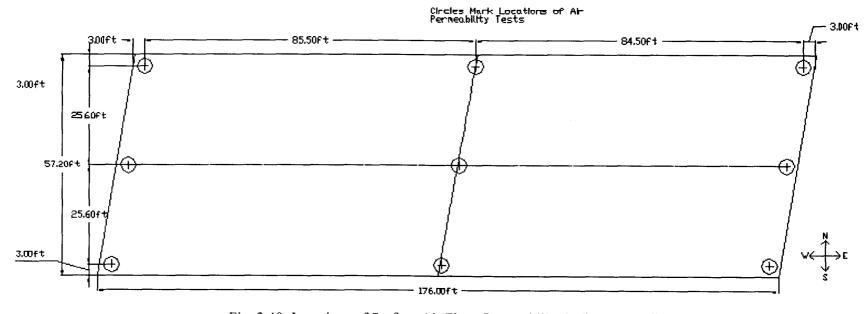
Fig. 3.40: Locations of Surface Air Flow Permeability Indicator Readings Route 130 Westbound
