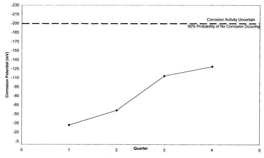
Fig. 4.11: North Main Street Eastbound GECOR 6 Average Corrosion Potential (mV)
