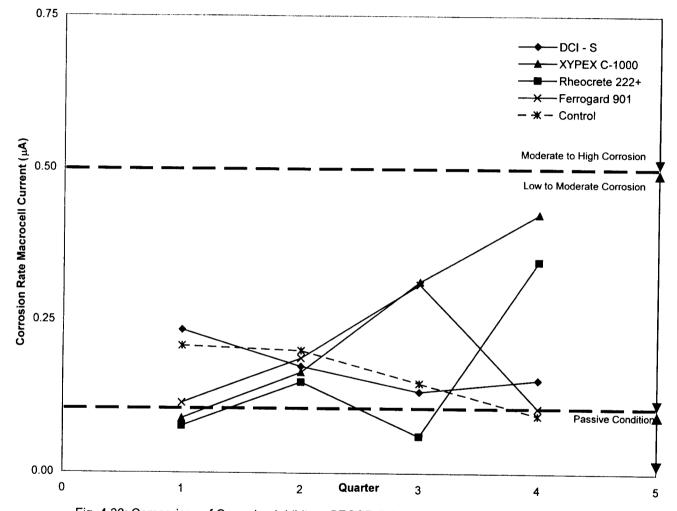
Fig. 4.38: Comparison of Corrosion Inhibitors GECOR 6 Average Corrosion Rate Macrocell Current (µA)
