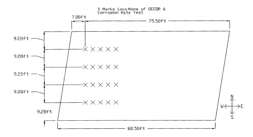
Fig. 3.13: Locations of GECOR 6 Corrosion Rate Meter Tests Wyckoff Road Westbound
