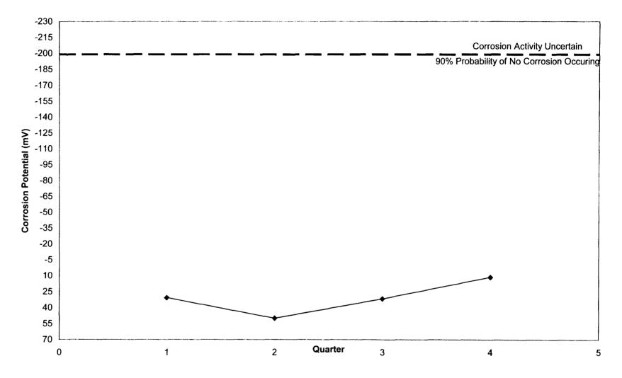
Fig. 4.32: Route 130 Westbound GECOR 6 Average Corrosion Potential (mV)
