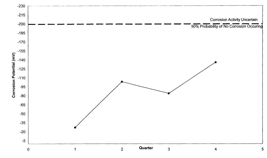
Fig. 4.18: Wyckoff Raod Westbound GECOR 6 Average Corrosion Potential (mV)
