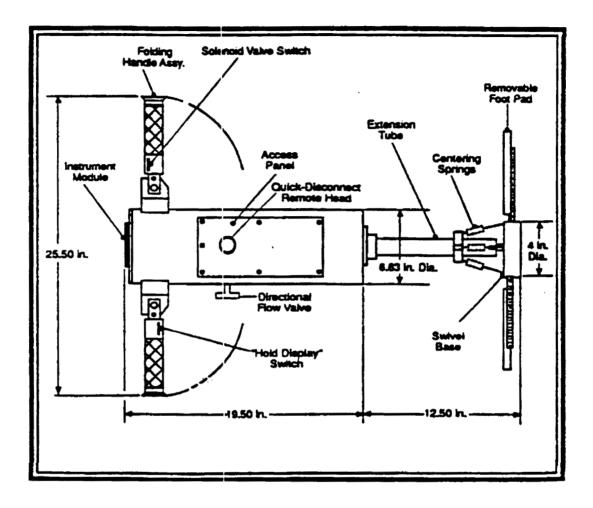
Fig. 3.6: Drawing of Concrete Surface Air Flow Permeability Indicator
