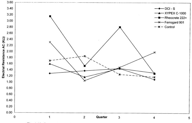
Fig. 4.40: Comparison of Corrosion Inhibitors GECOR 6 Average Electrical Resistance AC (K $\Omega$ )
