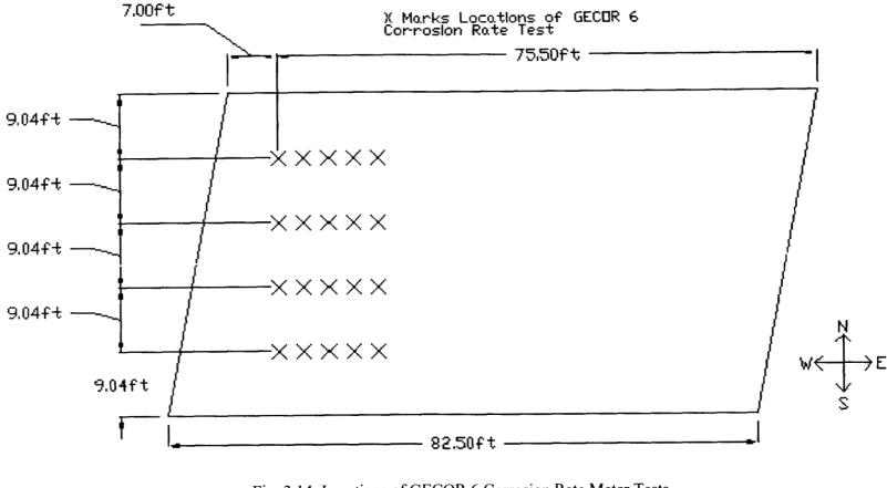
Fig. 3.14: Locations of GECOR 6 Corrosion Rate Meter Tests Wyckoff Road Eastbound
