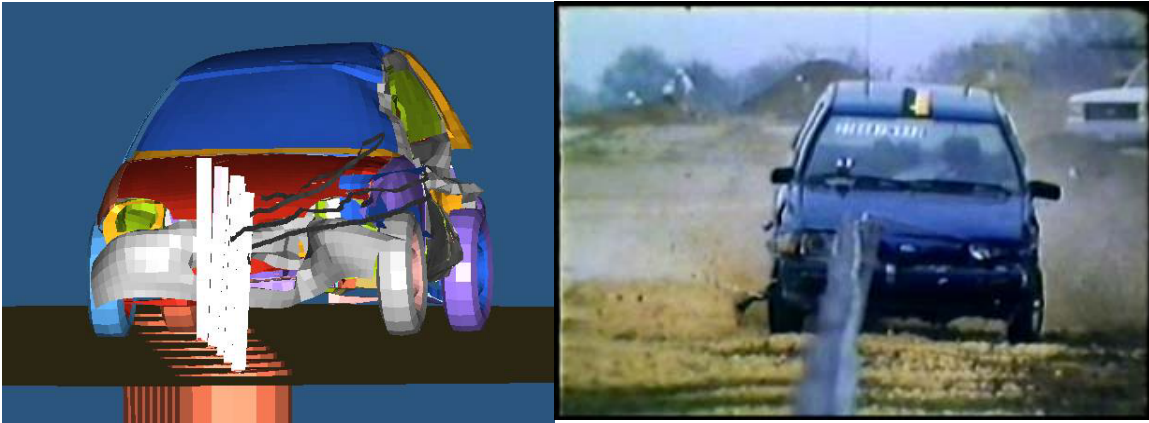
Figure 29. Three Strand Cable Barrier Validation: Model and Crash Test
