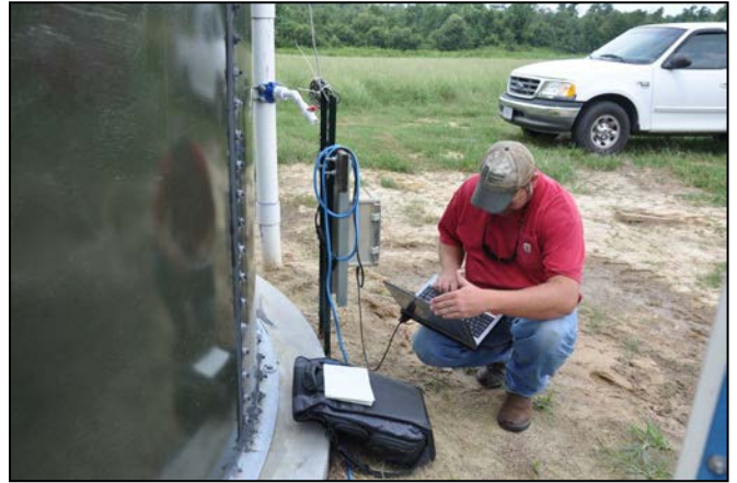
Picture at left shows box containing data-logger used to monitor plant liquid levels, temperatures, rain, pH and DO. Picture at right shows evaluation team member downloading data from a Doppler flow meter during weekly visits.
