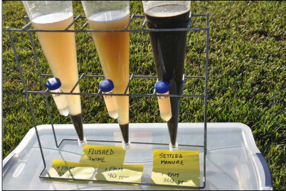
Figure 7. The two cones at left are flushed swine manure from the sow farm after 30 minutes settling in the laboratory (Table 12). The cone at right is settled sludge from decanting tank. The small vials are the effluents after polymer application and screening (Tables 13 and 14).
