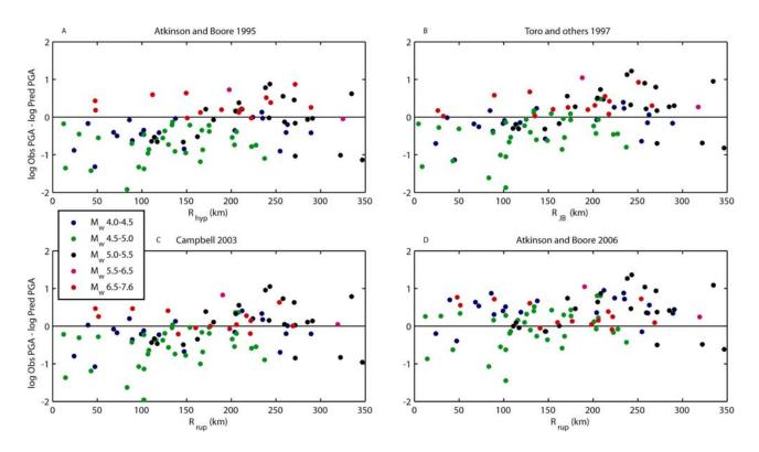
Figure 11. Residuals for the stable continent GMPEs against the global PGA dataset. Individual data residuals are plotted, color-coded by earthquake magnitude. The Atkinson and Boore (2006) GMPE for BC site classes is computed for a stress parameter of 140 bar.
