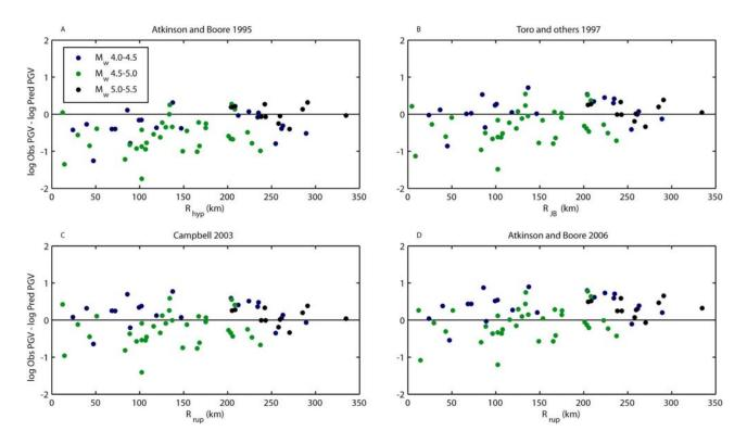
Figure 12. Residuals for the stable continent GMPEs against the global PGV dataset. Individual data residuals are plotted, color-coded by earthquake magnitude. The Atkinson and Boore (2006) GMPE is computed for a stress parameter of 140 bar.
