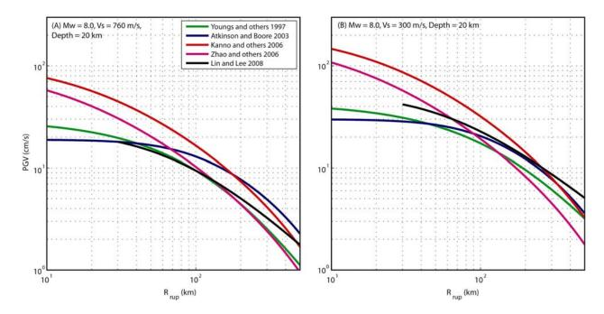
Figure 10. Amplitude-distance comparisons for the candidate subduction-zone GMPEs for an earthquake of magnitude  $M_W$  8.0 and focal depth of 20 kilometers, on (A) rock and (B) soil, respectively.
