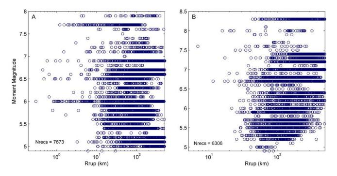
Figure 1. Magnitude-distance distribution of global PGA dataset gathered for the Atlas of ShakeMaps for (A) active crustal regions and (B) subduction zones. Only data recorded at distances *R*<sub>rup</sub> 500 kilometers and less are indicated.
