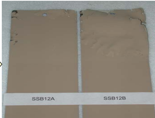
Solvent-borne System 53022B Primer / 53039 Topcoat
