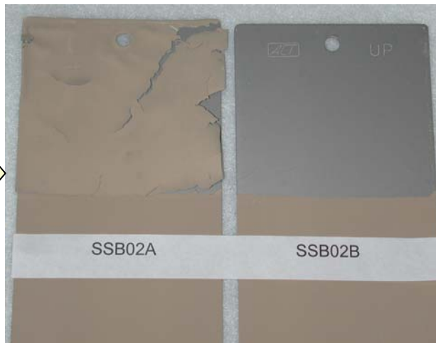
Solvent-borne System 53022B Primer / 53039 Topcoat
