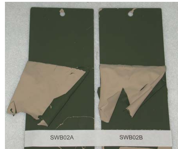
Water-borne System 53030 Primer / 64159 Topcoat
