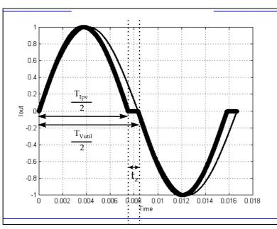
Figure 7. Example of a Waveform Used to Implement the Frequency Bias Method of Islanding Detection. A Pure Sine Wave is Shown for Comparison.
