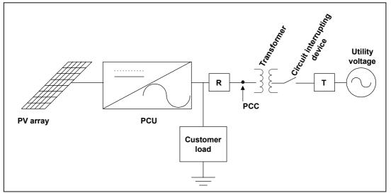
It is possible to use an existing utility PLCC signal for islanding prevention, without interfering with its normal utility use and without decoding the information in the signal. The PLCC methods are currently used to load shed with signals sent from
