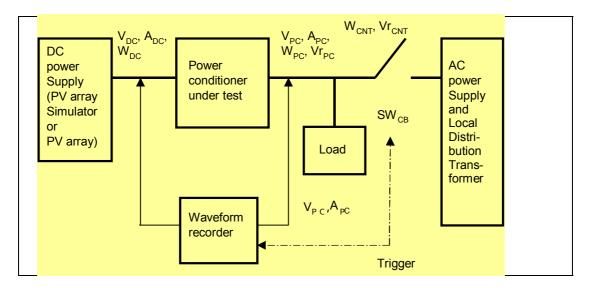
Figure 12. Suggested Anti-island Test Circuit in the DRAFT of the International Electrotechnical Commission Standard IEC 62116.
