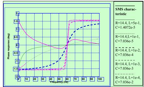
Figure 6. SMS Phase Response Curve and RLC Load Frequency Responses [1]
