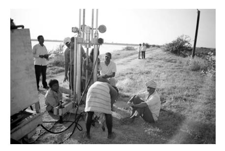
Figure 7c CPT test in progress
