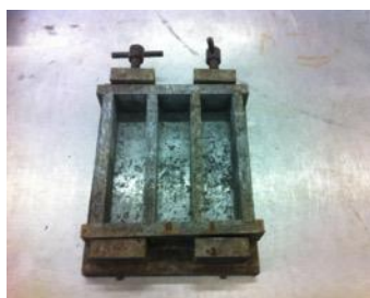
Figure 2 Standardized prismatic specimens molds
