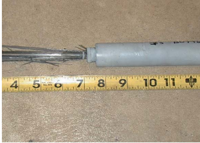
(a) Failure mode 1 (tensile-rupture)
