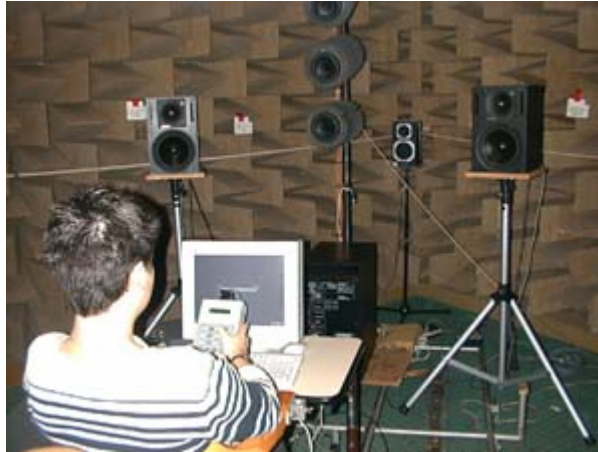
Figure 2.6. Psychoacoustics test in an anechoic chamber.
