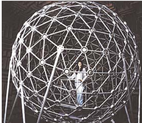
Figure 2.7. The sound localization facility at Wright Patterson Air Force Base in Dayton, Ohio, is a geodesic sphere, nearly 5 m in diameter, housing an array of 277 loudspeakers. Each speaker has a dedicated power amplifier, and the switching logic allows the simultaneous use of as many as 15 sources. The array is enclosed in a 6 m cubical anechoic room: Foam wedges 1.2 m long on the walls of the room make the room strongly absorbing for wavelengths longer than 5 m, or frequencies above 70 Hz. Listeners in localization experiments indicate perceived source directions by placing an electromagnetic stylus on a small globe.
