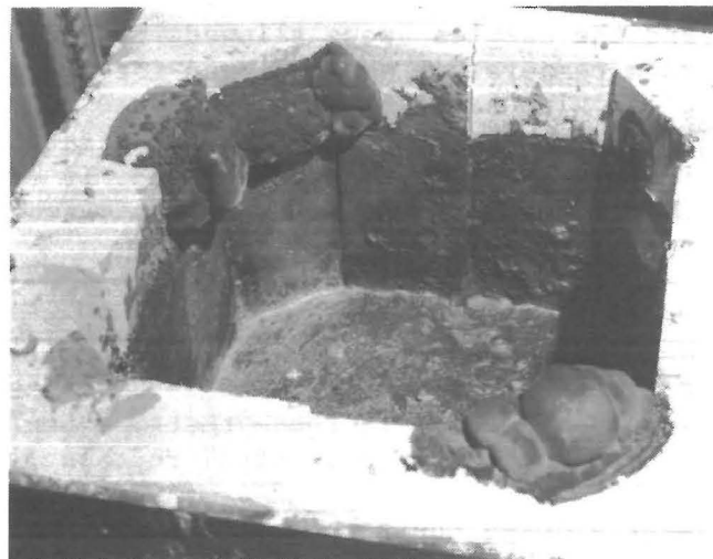
FIGURE 3.--Corundum formation on some refractory samples after 30-day exposure.
