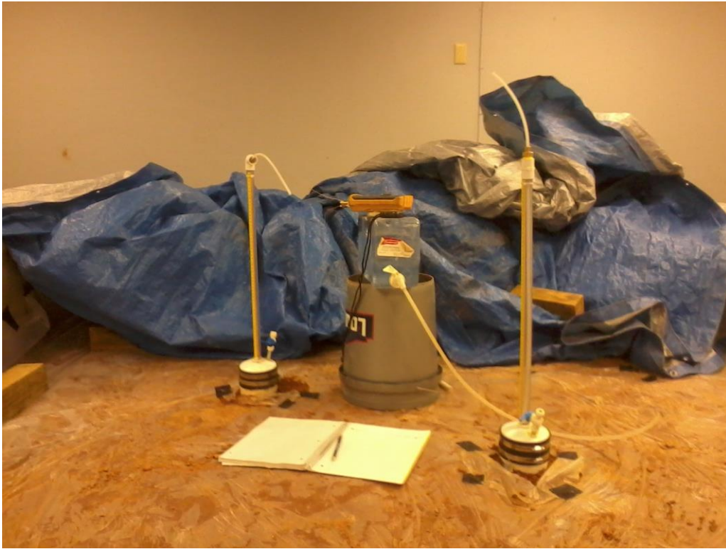
Fig. 8. Constant head TSB apparatus and TEG apparatus during testing (photograph taken by author).
