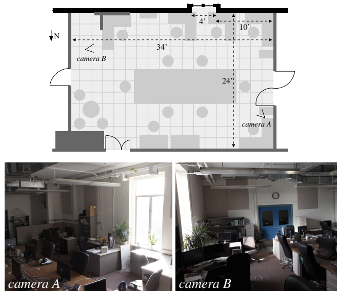
Figure 3: User study participants visited this simple open office environment as a case study for daylighting analysis. The room contains a single, tall and narrow, south-facing window that provides direct overly-intense illumination to portions of the room while leaving other areas relatively dark. Thus, occupants of the space typically turn on the overhead lights, and on sunny afternoons a diffusing shade is needed to prevent glare.
