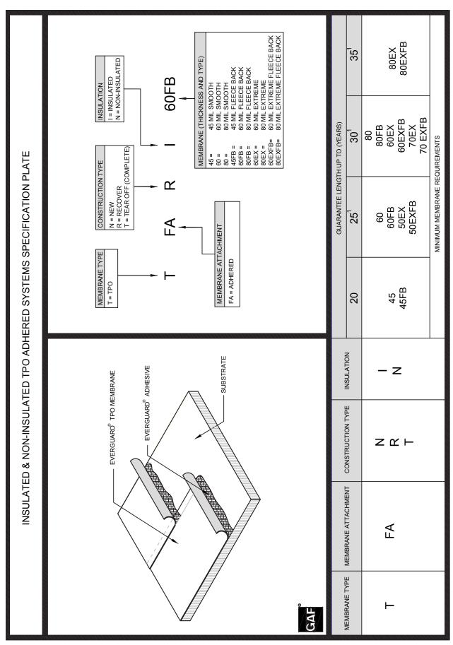
1. New & Tear-off only. Minimum 2 layers of insulation. Refer to the Guarantee Requirements Table for additional requirements on extended-length guarantees.
