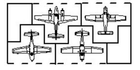
The standard configuration is sometimes called "stacked" because the unit depth is equal to the building width and the units are stacked together. Since the hangar width is narrower, it is also longer than the nested configuration thereby requiring longer taxi lanes on both sides of the hangar.
