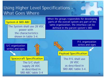
Figure 4: When the interface is defined in the parent system's SRD
