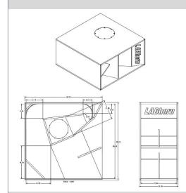
Schematics of the LAB Sub, a horn-loaded design developed by the PSW Live Audio Board community.
