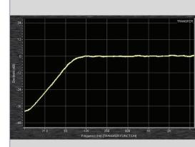
A 75 Hz high-pass filter from an input channel of a Mackie 1402 mixer as measured in transfer function mode on Rational Acoustics Smaart software. The filter has a slope of 18 dB per octave.
