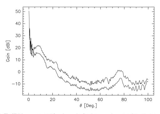
Figure 9: The VLA beam out to 100° from bore-sight. Simulation was done at 1.5 GHz. The bottom curve shows the azimuthally averaged gain at the given value of  $\theta$ . The top curve shows the maximum gain at the given angle. Note the peaks near 20 and 75° that arise from reflections off the struts. The smooth bump from 5 to 15° comes from feed spillover around the subreflector.
