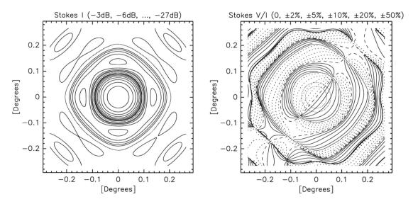
Figure 8: The VLA beam pattern at 8.4 GHz out to the second sidelobe shown in total power (left) and fractional circular polarization (right). The red contours show the first two beam nulls. The green contours show -3dB and -6dB total power. A feed position angle of  $140^{\circ}$  was used. Stokes Q and U are not shown since the coarse gridding (required by time constraints) made for suspicious linear polarization plots.
