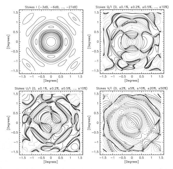
Figure 2: The VLA beam pattern at 1.53 GHz out to the second sidelobe shown in total power (Stokes I) and fractional polarization. The red contours show the first two beam nulls. The green contours show -3dB and -6dB total power. A Gaussian feed with a -12dB taper at 9° feed angle, a good approximation to the EVLA L-band feed, was used. The feed was located at  $-135^{\circ}$  in the feed circle, half way between two struts.
