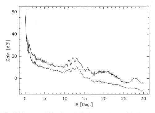
Figure 11: The VLA beam out to  $30^{\circ}$  from bore-sight. Simulation was done at 5 GHz. The strut feature is present at 17 to  $23^{\circ}$  and the feed spillover feature is seen from 11 to  $13^{\circ}$ .
