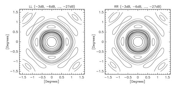
Figure 4: The VLA beam at 1.53 GHz in Left (LL=I-V) and Right (RR=I+V) polarizations. Superimposed on these plots are green contours showing the -3 and -6dB total power contours and red contours showing the first two nulls. Note the beam squint that separates the LL and RR beams. The squint is more easily seen in the 1-D beam cuts of Figure 5. As for Figure 3, the Stokes V data were antisymmetrized before computing the LL and RR beams.
