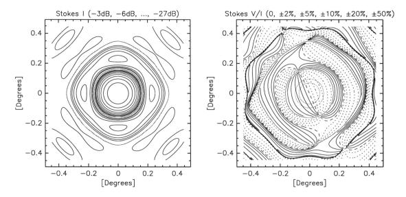
Figure 7: The VLA beam pattern at 5 GHz out to the second sidelobe shown in total power (left) and fractional circular polarization (right). The red contours show the first two beam nulls. The green contours show -3dB and -6dB total power. A feed position angle of 25° was used. Stokes Q and U are not shown since the coarse gridding (required by time constraints) made for suspicious linear polarization plots.
