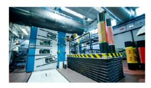
Given the larger printing repeat range provided, and the higher dimensions of its framework, all presses in this series are equipped with the optional "SRS" Smart Ride System with special sleeve trolleys and lifting platforms for quick access to the upper printing units. That makes handling sleeves for big repeats easier, as well as sleeve change.
