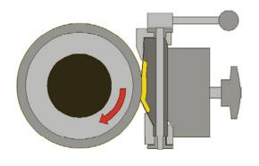
New doctor blade chamber with innovative design by Koenig & Bauer Flexotecnica
