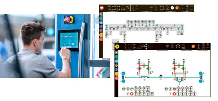
**ErgoTronic** is the name of the new control system for Koenig & Bauer Flexotecnica printing presses featuring completely new PLCs, motion logic drives and high quality industrial operator panels to achieve increased system performance, accuracy and reliability.
