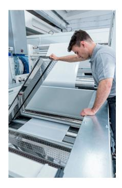
The new drying tunnel is equipped with panels featuring an array of high-efficiency, deep-drawn circular holes which can be easily removed from the operator side for cleaning. They are specially designed to reduce air pressure loss and ensure maximum air turbulence at high printing speeds.
