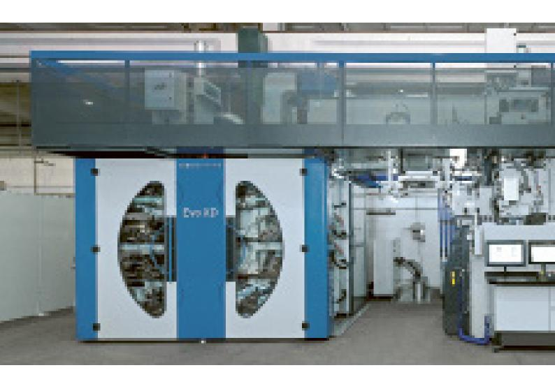
The machine layout shows a "versatile" configuration so to enable the application of any print technology, either solvent- or water based, in this way keeping the machine investment away from any future technological obsolescence.
