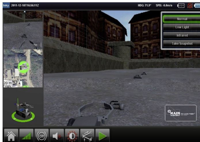
Figure 2. An early user interface design for AEODRS. The display configuration is designed for a small handheld OCU to control a small tracked vehicle with a manipulator. The small windows on the left can be swapped into the main area on the right to enable a larger view of the content. The tiled display with temporary overlays was chosen to minimize content obstruction.
