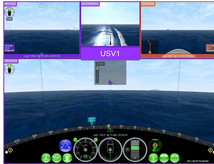
Figure 3. A display developed for an ONR effort to safely and efficiently control multiple USVs navigating a congested environment. The USV's video display is arranged to provide the operator with better spatial and situational awareness and a forward view from a second USV is in constant view. Most of the operator's interaction is by a standard gamepad, reducing training requirements for basic control substantially. All but the video and maps are HTML including the window borders, gauges, and text gauges. Parts of the display are many layers thick drawn by multiple modules, but display as one common interface.
