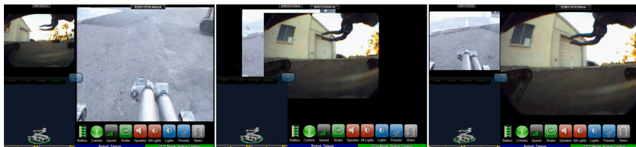
Figure 1. This display configuration allows one of three windows to be displayed in the larger location. The windows are animated between locations to show the user which screens are exchanging position. This example shows three screenshots while the user chooses an enlarged drive camera in place of a payload camera.
