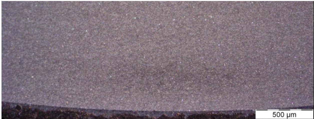
Figure A-3. Micrograph of the RCF affected region of the Ball #14 after chemical etching.
