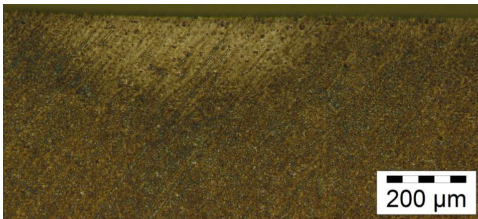
Figure A-12. Micrograph of the RCF affected region of the rod track #17 after chemical etching.
