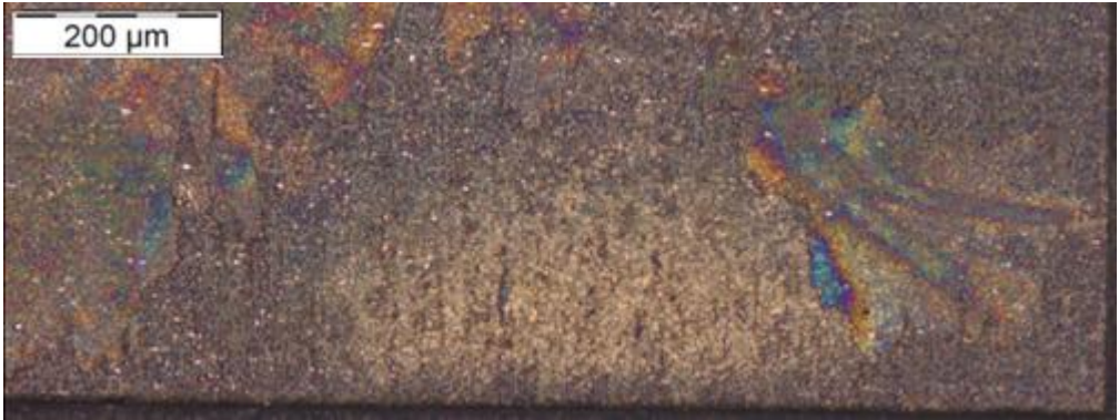
Figure A-16. Micrograph of the RCF affected region of the rod track #22 after chemical etching.
