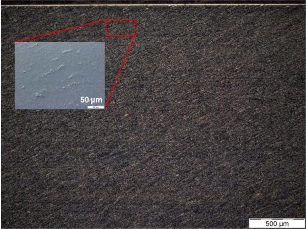
Figure 1-5. Distribution and size of carbides in M50 bearing steel.
