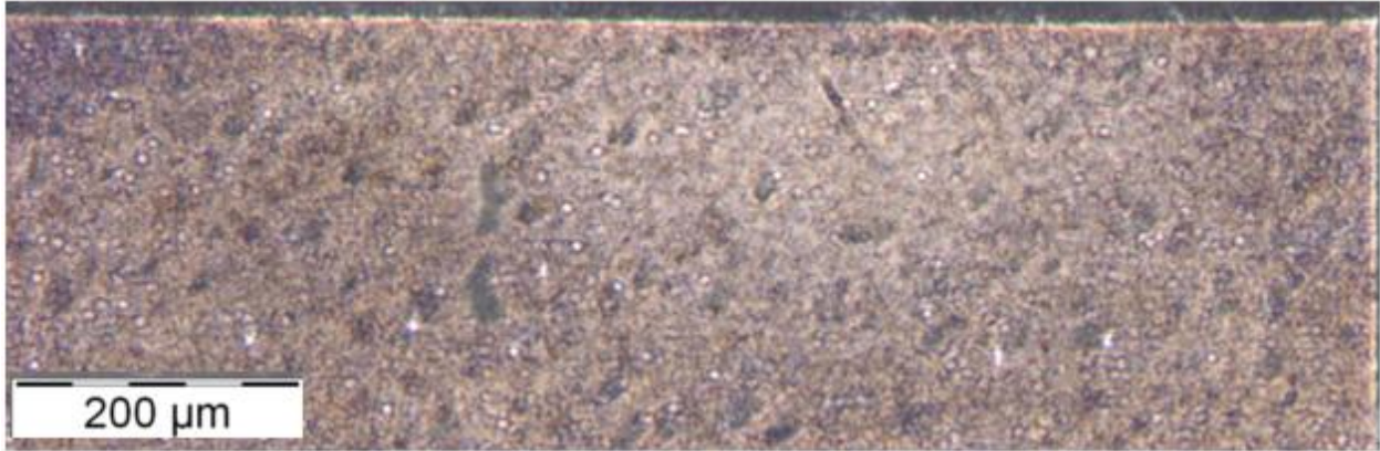
Figure A-17. Micrograph of the RCF affected region of the rod track #26 after chemical etching.
