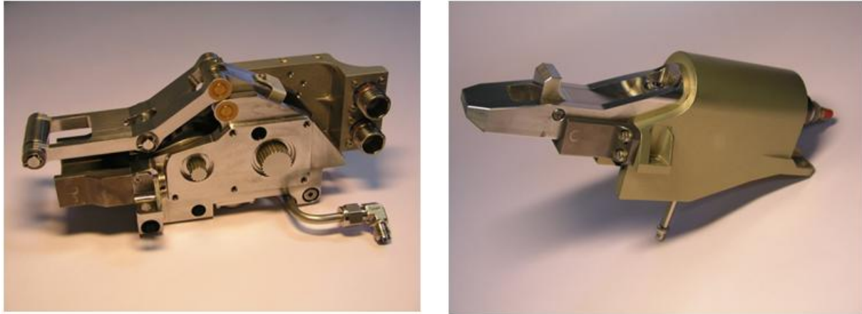
Figure 2 The Latch (left) and Latch Tab (right) of the first generation latching system
