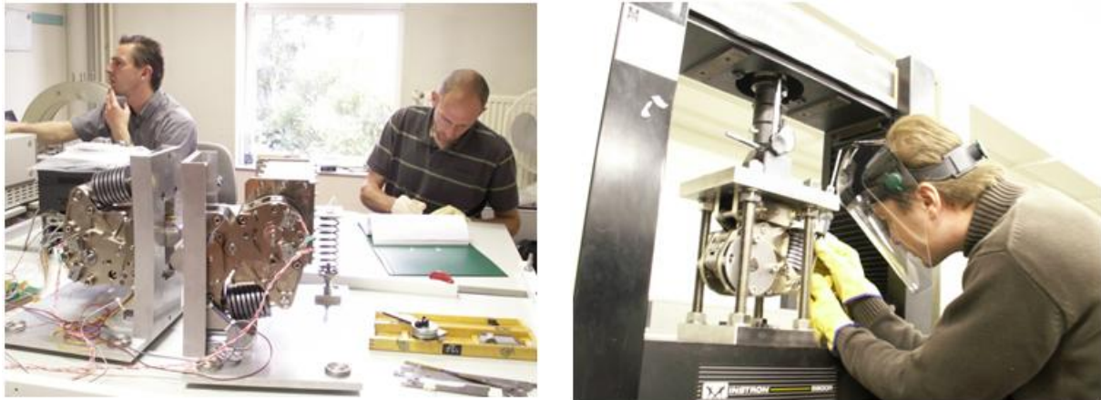
Figure 4 Functional and structural testing of the second generation latching system
