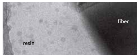
4 % nanosilica – TEM-Pictures of GFRCs with different levels of SiO 2 -nano-particles (based on NANOPOX® F 400)
