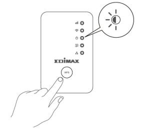
2. Wait for the extender to restart. The extender is ready for setup when the green power LED displays on.
