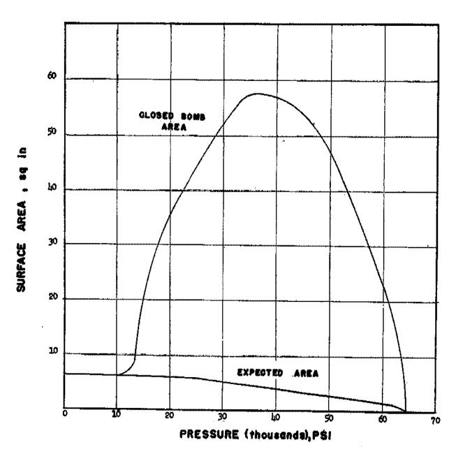
EXPECTED SURFACE AREA VS ACTUAL AREA OBTAINED FOR COMPOSITION B CYLINDER BURNED IN CLOSED BOMB
