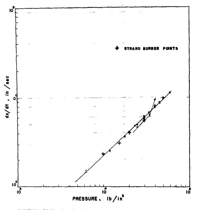
LINEAR BURNING RATES OF A R P PROPELLANT OBTAINED WITH CLOSED BOMB AND STRAND BURNER UNCLASSIFIED
