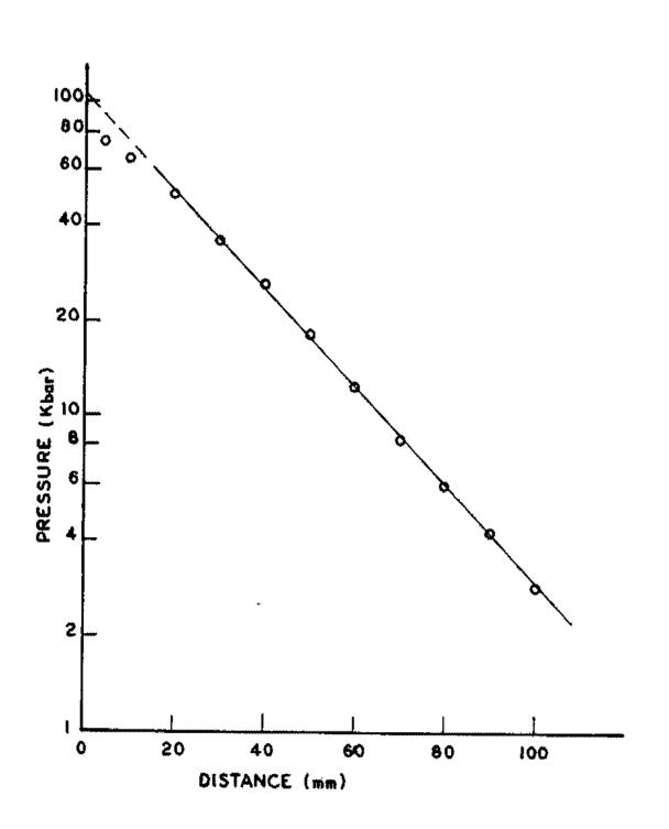
FIGURE 4. Log of Pressure versus Distance in Lucite, loaded as in gap test.
