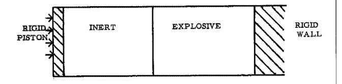
FIGURE 6. One Dimensional Model For Theoretical Treatment of Gap Test. Rigid Piston at Left Compresses Inert Material and Explosive Against Rigid Wall at Right.
