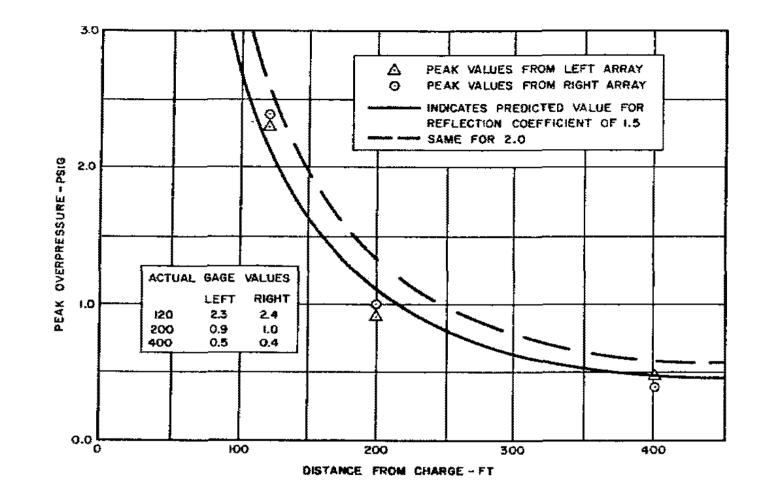
Figure 4. Calibration Test No. FC-1A Pad 3 for Minuteman Charge 100 Pounds Comp. C Fired 6 January 1960.
