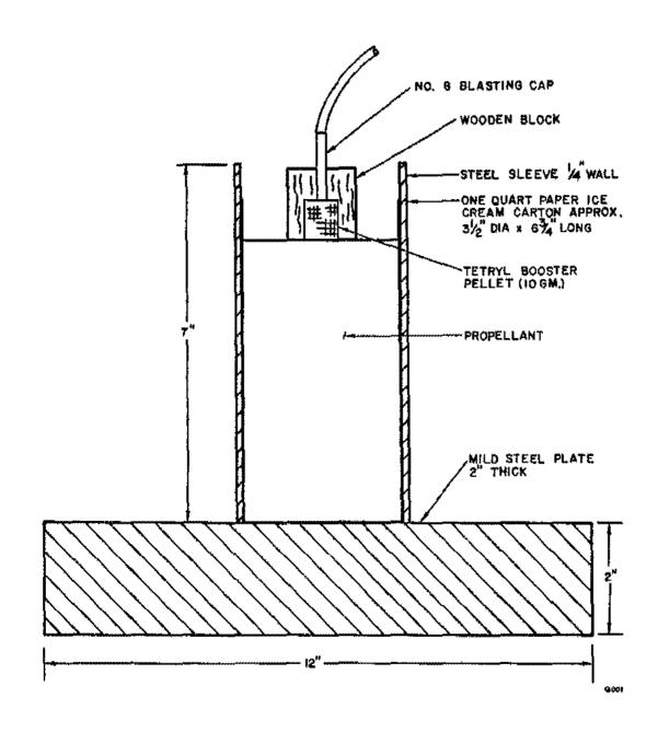
Figure 1. Section View of Field Explosive Test Setup for Susceptability to Detonation Tests.
