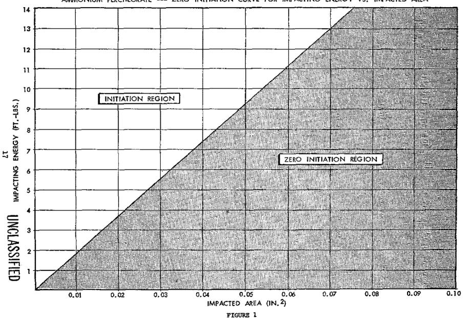
AMMONIUM PERCHLORATE --- ZERO INITIATION CURVE FOR IMPACTING ENERGY VS. IMPACTED AREA
