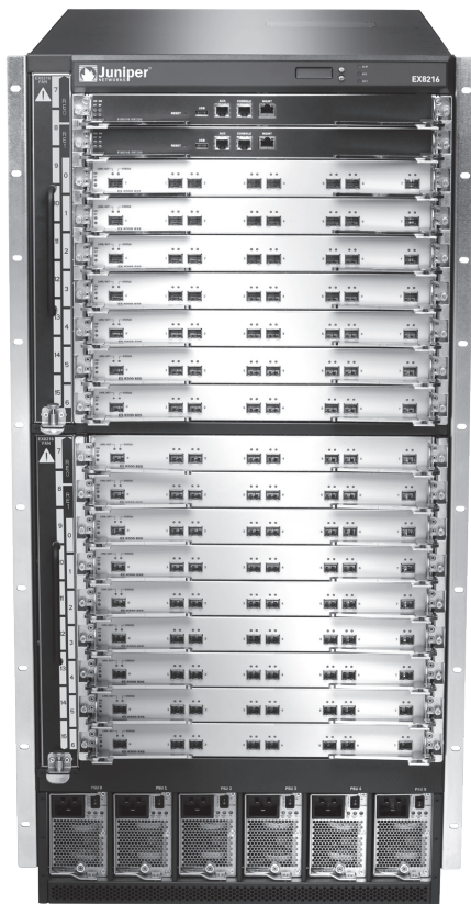
The EX8200 line of switches delivers high-speed, high-density platforms for aggregation and core deployments.
