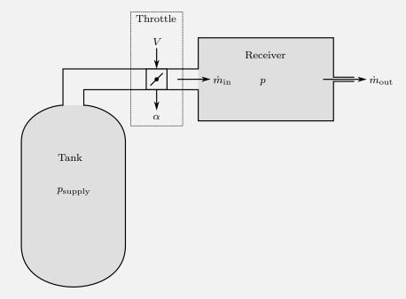
You have installed sensors to measure the pressure p in the receiver as well as the position  $\alpha$  of the throttle valve. The voltage V is applied to the electronically controlled throttle and  $\dot{m}_{\rm in}$  is the mass flow into the receiver. The following control architecture is to be used.
