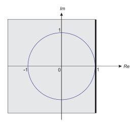
Using the same reasoning, it can be shown, that both the Euler Backward and the Tustin transformations map the entire stable continuous-time pole region to the stable discrete-time pole region, thereby maintaining controller stability.
