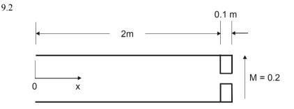
The tube shown in the figure above is terminated at the right end by an orifice plate. At 200 Hz, sound introduced into the left end of the tube produces a standing wave in the tube which has a minimum located 0.2 m from the inside edge of the orifice when the temperature in the tube is  $20^{\circ}$ C.
