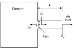
source is a fan located 10m upstream from the plenum chamber. The downstream ductwork is terminated in its characteristic impedance (such that no sound waves are reflected upstream from the termination). Define all impedances used in your expression and give numerical values to each quantity necessary to evaluate these impedances.
