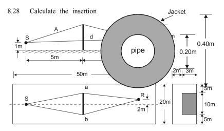
loss in octave bands between 63Hz and 8kHz due to wrapping a 200mm diameter steel pipe with a 100mm layer of 90kgm<sup>-3</sup> glass fibre covered with an aluminum jacket weighing 6kgm<sup>-2</sup>.
