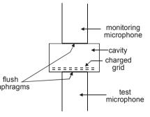
3.21 The acoustic coupler diaphragms shown in the figure at right can be used to determine the internal
