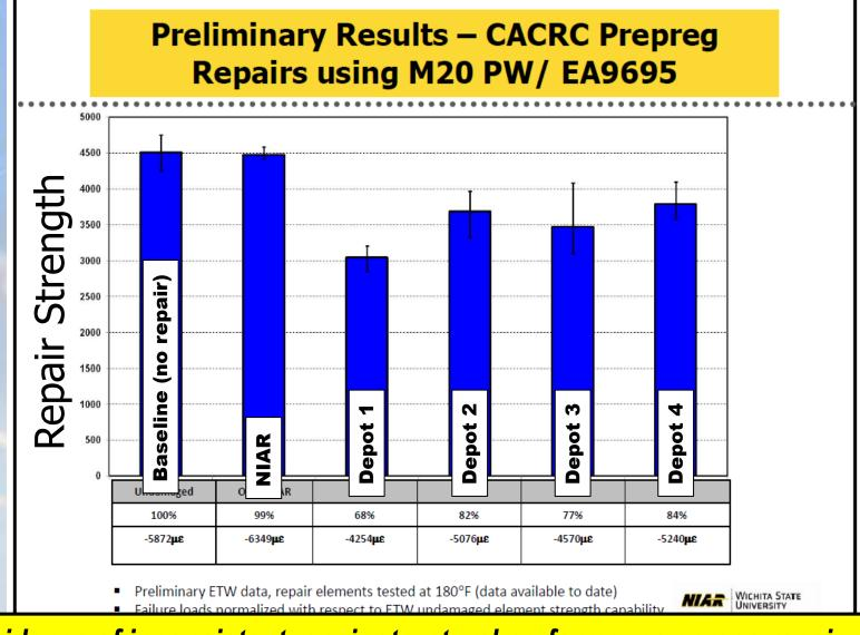
2014 evidence of inconsistent repair structural performance across repair depots (lowest regults show only 68% strangth restaration)
