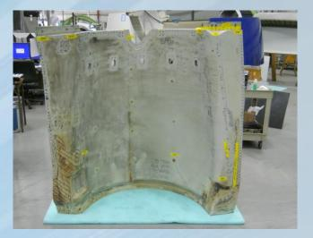
Compared Large Number of Damaged Inner walls: -Damage location was consistent -Damage area (size) was consistent -Found correlation between damage size and time on wing -From data, could categorize two basic geometry needs for a repair kit (Reviewed **more than 600 panels**)
