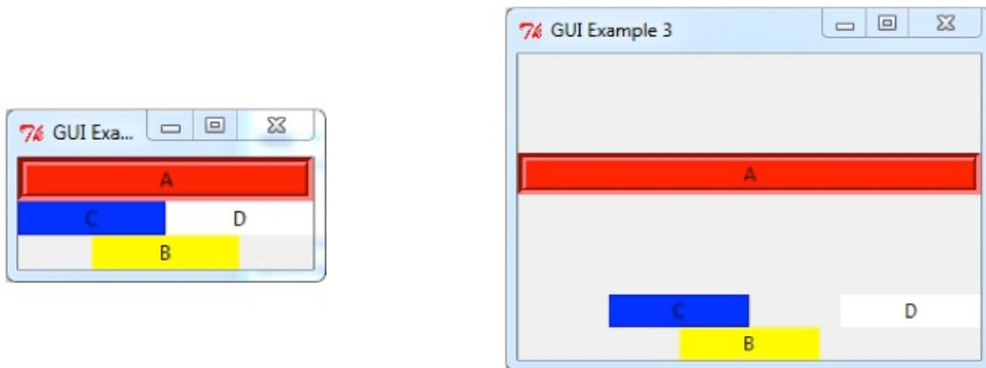
The desired behaviour is shown below. The four labels are positioned at the corners and the labels fill the space when the window is resized.
