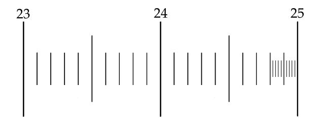
Fig. 2.2 - Stage Micrometer: On the metric scale, lines 1 - 25 are spaced exactly 1mm (1000μm) apart, the lines between 24 and 25 are spaced 0.1mm (100μm) apart, and the smallest lines (far right) are spaced 0.02mm apart. Note - 0.02 mm = 20 micrometers (20μm) = 20 microns = 20μ.
