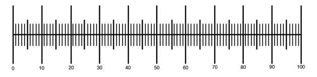
Fig. 2.1 - Ocular Micrometer: The distance between the lines is arbitrary, and changes when different objectives are being used.
