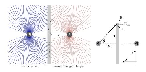
Figure 1: Left: The field of a charge near a conducting plane, found by the method of images. Right: Setup for calculating the field.
