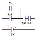
Using our rule for combining series capacitors, we can find the value of  $C_{84}$  easily:
