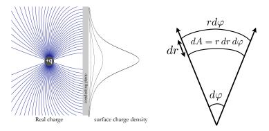
Figure 2: Left: Surface charge density as a function of the lateral position on the plate for various distances from the plate. Right: Element of area in polar coordinates.
