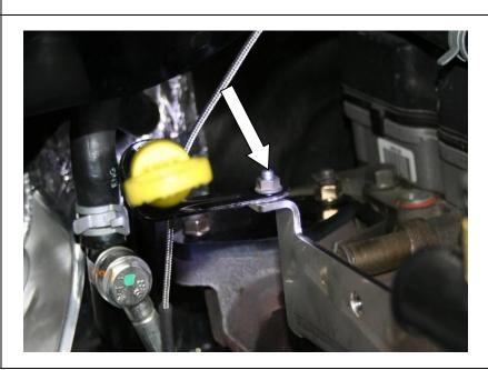
27.Reinstall the existing back pressure tube with the factory bolt onto the delete bracket & leave loose.
