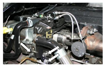
11.Remove the three bolts for the stepper motor bracket (10 mm) socket and prop the bracket on the cooler.
