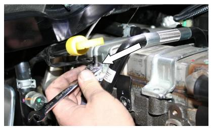
17. Remove the EGR coolant hose from the cylinder head to the cooler. (All bolts should be already removed) the hose is held in by O-rings. Remaining coolant will drip out.
