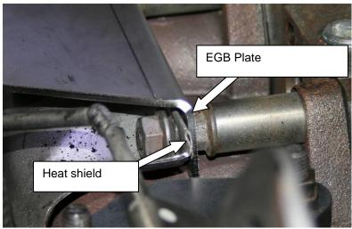
26.Install the transmission dipstick tube to the delete plate and torque to 89 in/lbs.
