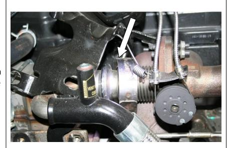
13.Using a (15mm) socket remove the outer nut for the exhaust flange of the flow valve at the manifold.
