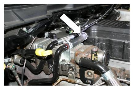
16. Remove the four bolts for the cooler and the nut that holds the transmission dip stick tube in place. Then nudge the tube out of the way to access the nut under the dip stick bracket.
