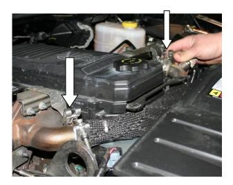
3. Loosen the cross over pipe clamps (11 mm) and slide them down the pipe. Remove the bolt located at the center of the pipe, and remove the pipe from the vehicle.
