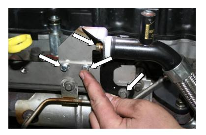
30. Tighten the plug bolt, then tighten the coolant hose bracket bolt to 89 in/lbs then the EGB bracket to 89 in/lbs also.
