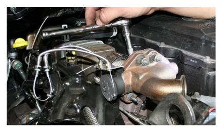
14. Remove the EGR flow direction valve from the vehicle.
