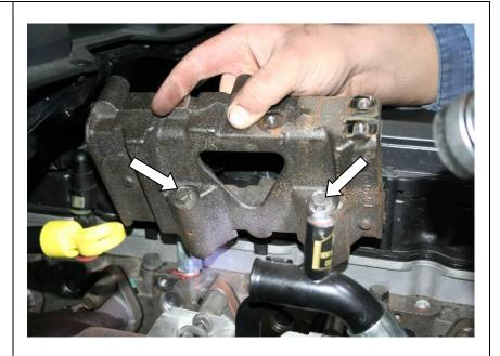
22. The supplied Back plate is drilled & tapped 1/8" NPT for a Pyro install. If there is no Pyro to be installed insert the supplied brass plug (1200208) and continue.
