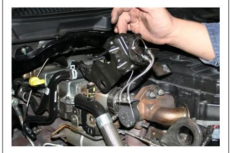
12.Loosen the clamp (11mm) that connects the EGR Flow Direction Valve to the cooler and slide the clamp towards the valve.
