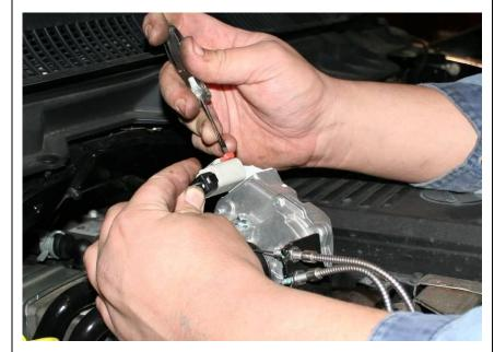
7. Next unplug the stepper (servo) motor connector and remove the two bolts (8mm) that hold the motor to the stepper motor bracket. Then release the cable to remove the motor from the vehicle.
