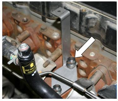
25.Loosen the top two manifold nuts about a 1/4". Install the EGB plate just behind the heat shield and tighten/torque the nuts (15mm) to 18 ft/lbs.
