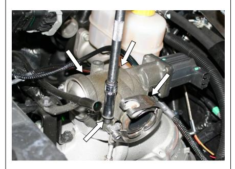
6. Install the EGB intake plates with the supplied gaskets to the intake horn reusing the existing hardware.
