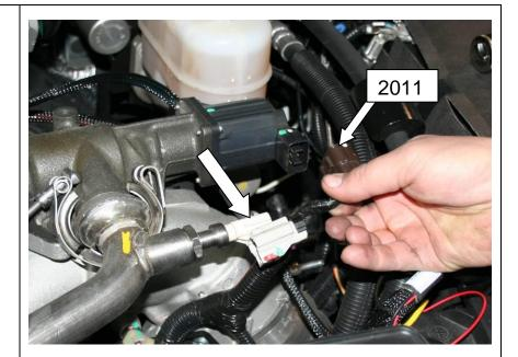
5. Remove the four bolts that secure the EGR valve to the intake horn (intake plenum) and remove the valve from the vehicle. (10mm)
