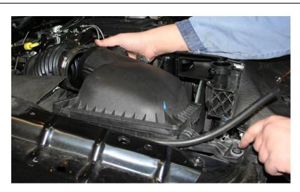
10.Remove the top bolt from the lower heat shield (10mm) then the other two (8mm) bolts to release the lower heat shield.
