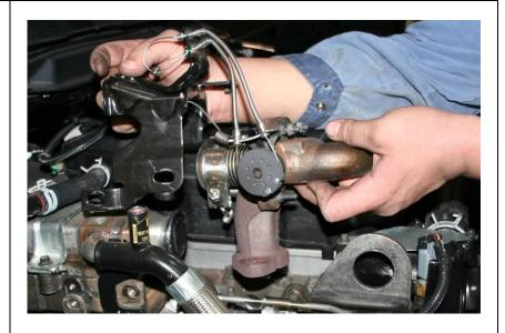
15.Remove the bolt that holds the CCV hose to the cooler then disconnect the clamp at the valve cover to remove the hose assembly.
