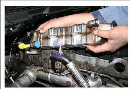
20.If the vehicle is a 07/08 insert the plug (1900036) into the coolant hose and tighten with the supplied gear clamp (1453113).
