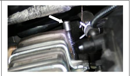
19. Prop the cooler above the studs and push towards the cab holding the other coolant hose to release the O-ring fitting to remove the cooler from the vehicle.
