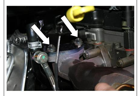
24.Install supplied Front Exhaust Plate (1900034), reusing the OEM Nuts, OEM gasket and the supplied (1405976) M10 spacer. Torque to 18 ft/lbs.
