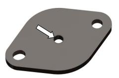
23.Install supplied Rear Exhaust Plate (1900033), reusing the OEM Nuts, OEM gasket and the supplied (1405976) M10 spacer. Torque to 18 ft/lbs.
