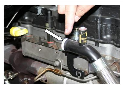
29.Install the accessory bracket starting with the coolant plug bolt then insert the other two bolts to secure the accessory bracket to the main bracket.
