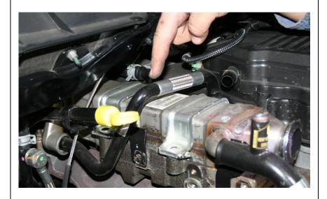
18. Remove the coolers two rear bolts that attach it to the exhaust system (15mm)
