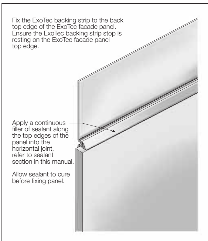
FIGURE 20 APPLYING SEALANT TO HORIZONTAL JOINT
