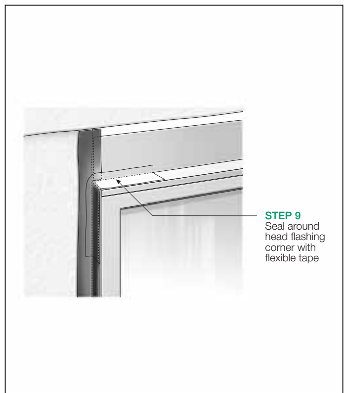
FIGURE 38 INSTALLATION OF WINDOW
