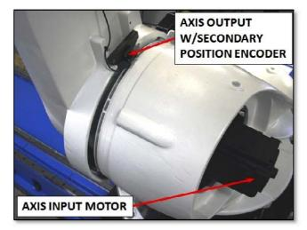
Figure 1. Robot axis with secondary encoder
