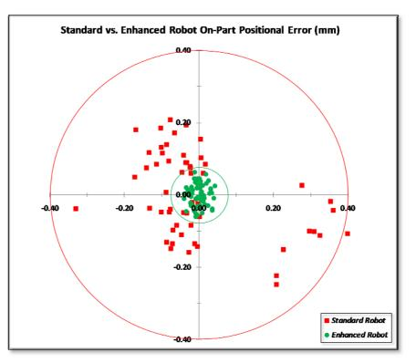
Figure 7. On-Part Accuracy Comparison
