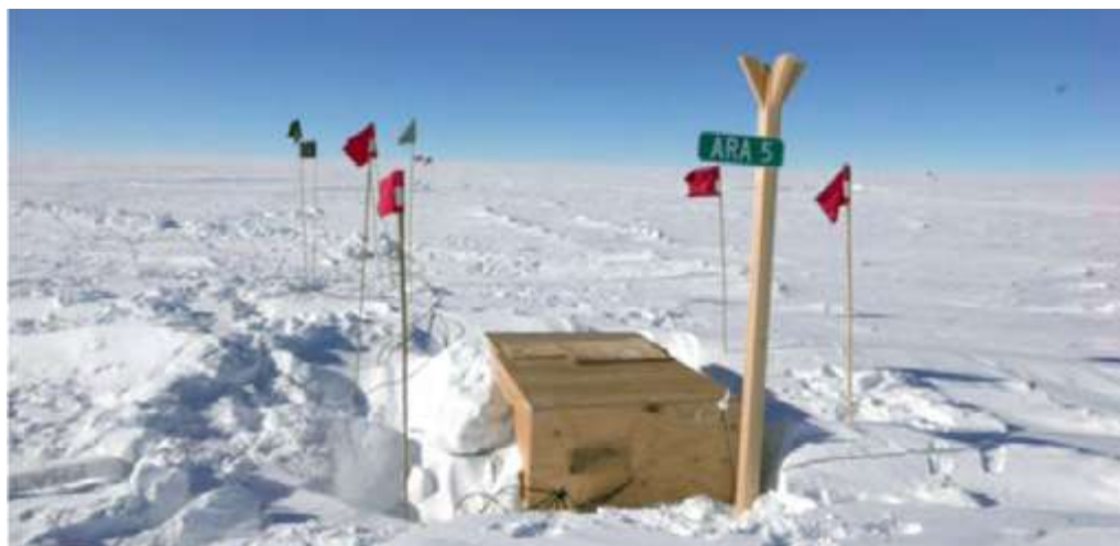
Part of the Askaryan Radio Array near the South Pole, the phased array detector makes finding possible neutrino-creating events easier. Here the detector's antenna extends above ground.
