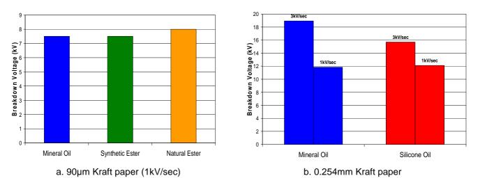
Figure 4.4 – Breakdown voltages of impregnated Kraft paper
