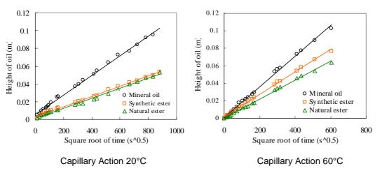
Figure 9.2 – Graphs of Capillary action at 20°C and 60°C
