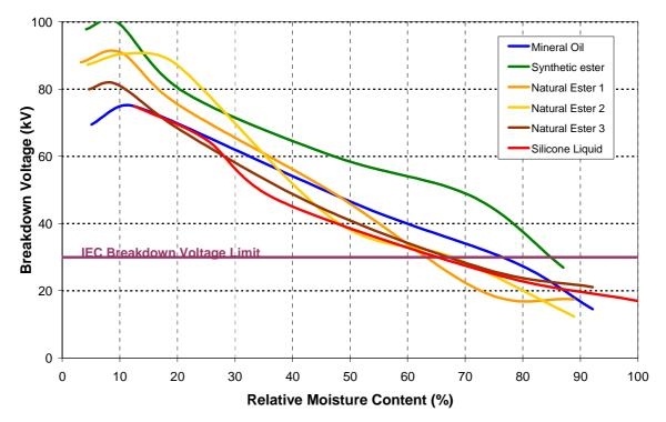
Figure 4.2 – Effect of relative moisture content on AC breakdown strength of fluids
