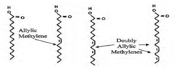
Figure 3.11 - Types of unsaturation found in natural ester fatty acid chains (Source: CARGILL)
