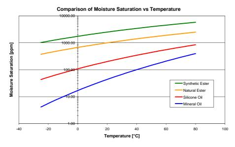
Figure 3.8 – How moisture saturation varies with temperature
