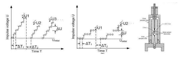
a. 1 shot/step rising-voltage method b. 3shots/step rising-voltage method c. test cell Figure 4.7 – Impulse breakdown voltage test method and electrode configurations
