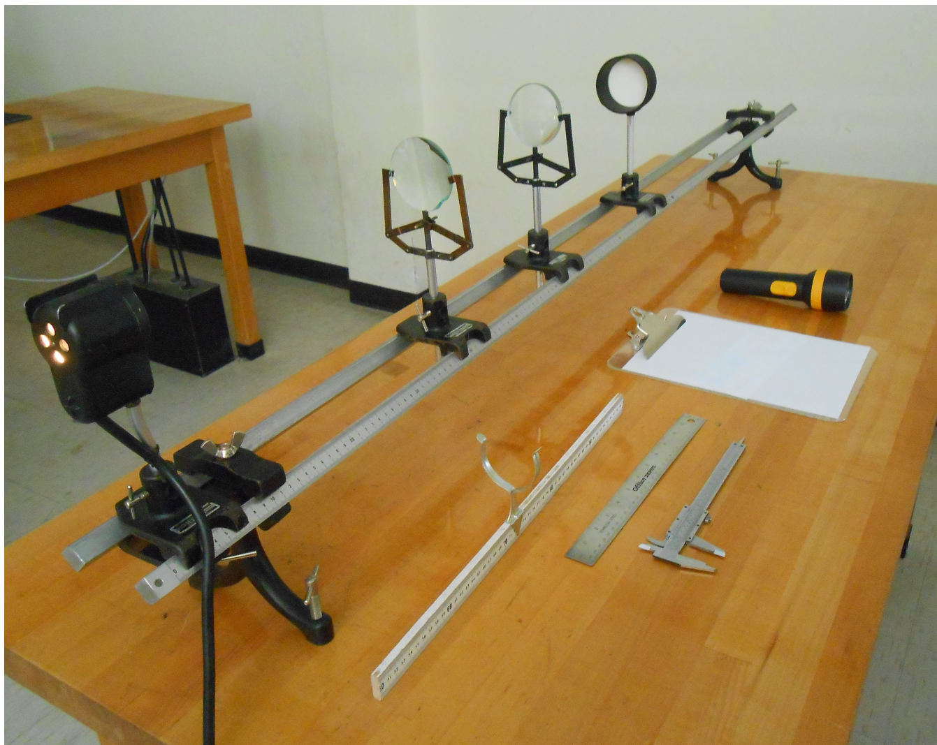
Figure 20.1: Optical Bench Arrangement
