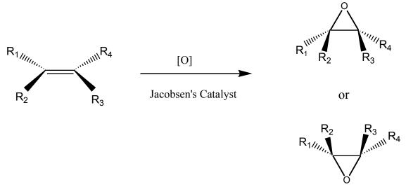
In Jacobsen's systems, the stereoselectivity relies solely on nonbonded interactions, thus lifting the requirement for a pre-coordinating pendant group (such as the alcohols above). In fact, alkyl- and aryl-substituted olefins react with Jacobsen's systems to give the highest enantioselectivity yet realized for nonenzymatic catalysts.
