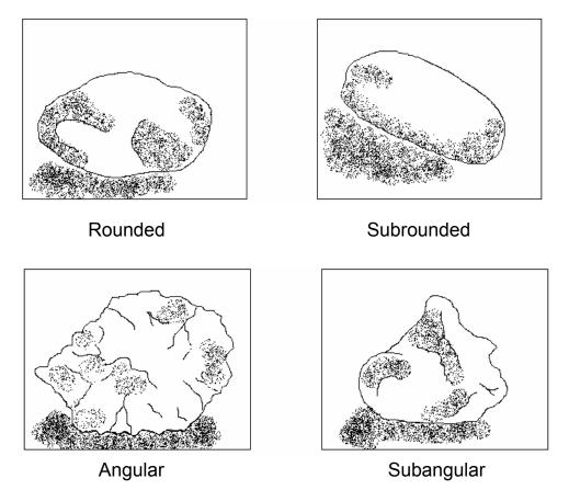
Figure 1. Shape of Coarse-Grained Soil Particles
