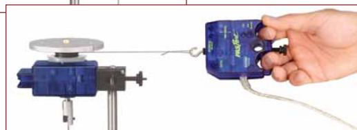
To determine the torsional spring constant, a torque is applied by pulling with a Force Sensor.
