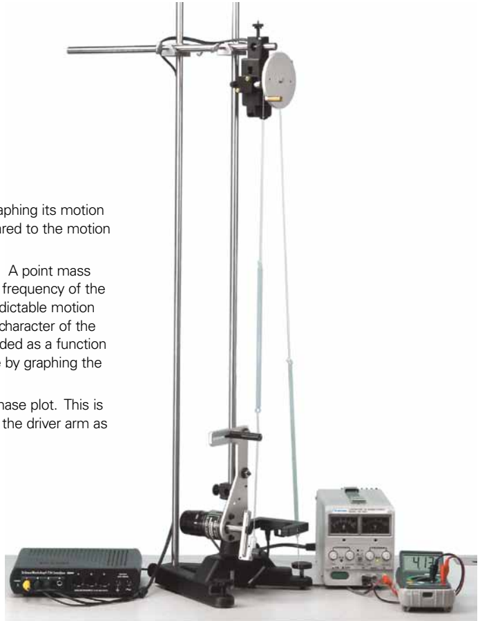
A graph in phase space and a Poincare plot are obtained to study the chaotic motion of this nonlinear oscillator.
