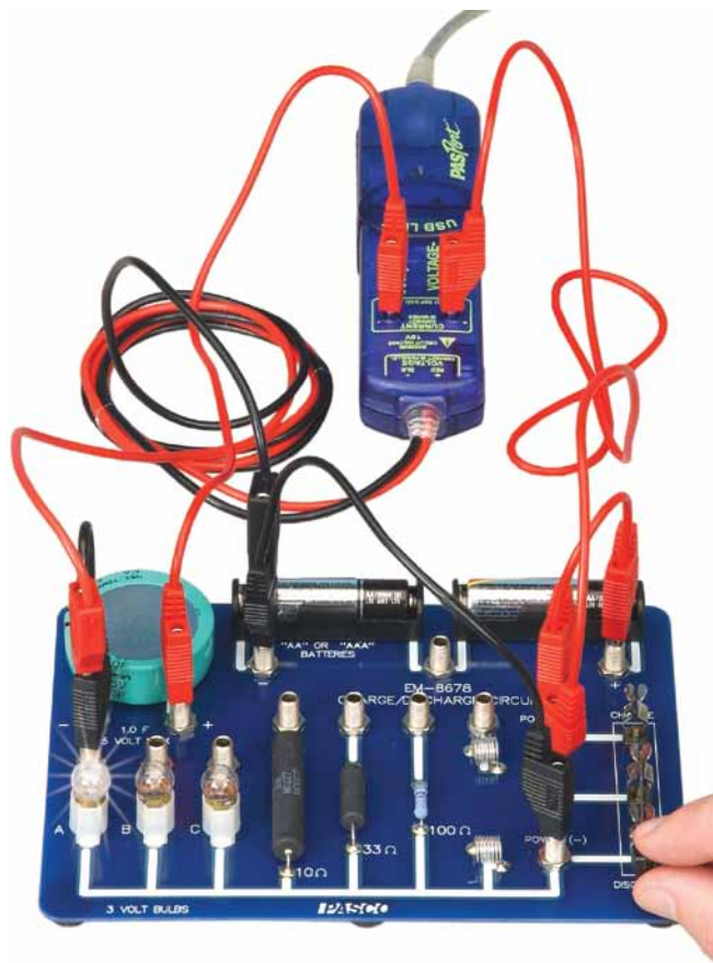
Voltage across and current through the light bulb are measured real-time as the capacitor discharges.
