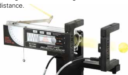
Two photogates are mounted at a fixed distance apart on the Projectile Launcher to measure the initial speed of the ball
