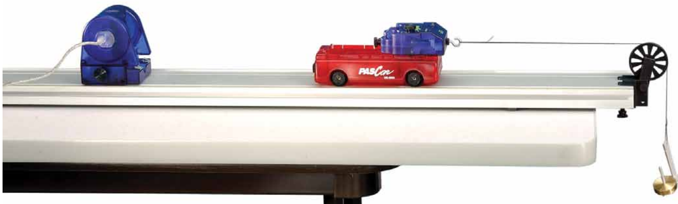
Students can effectively study Newton's Second Law with a Dynamics System, Force Sensor and Motion Sensor.
