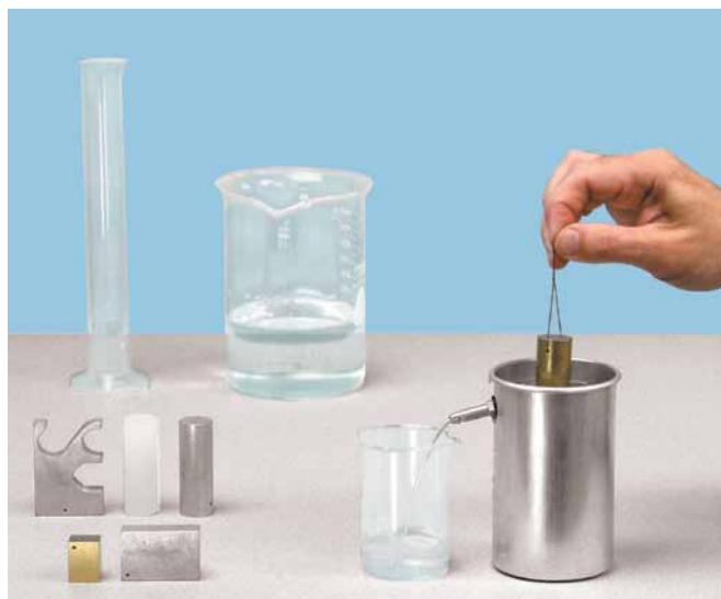
The buoyant force is measured by weighing the water displaced by the object.
