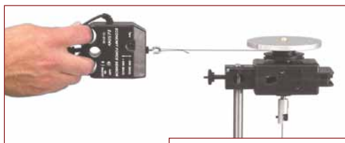
To determine the torsional spring constant, a torque is applied by pulling with a Force Sensor.
