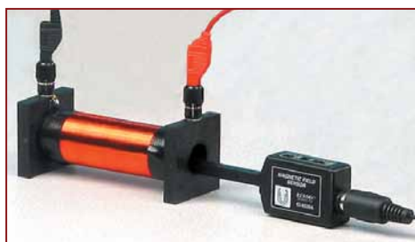
The magnetic field inside a solenoid is measured in the radial and axial directions.
