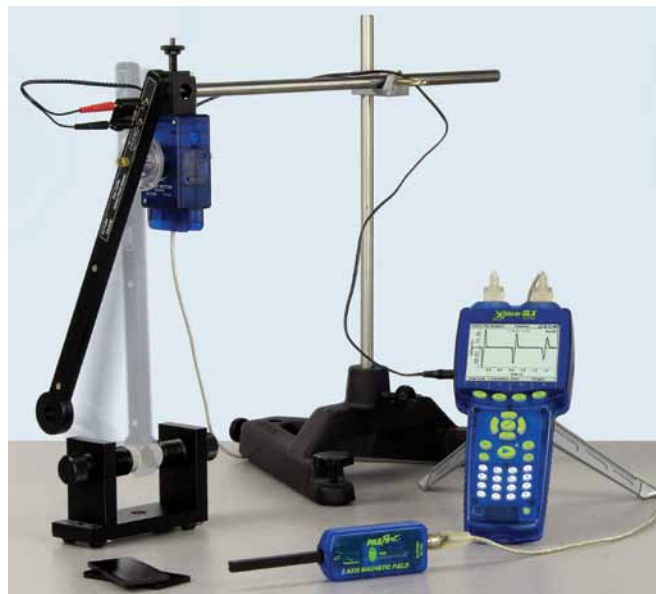
A voltage is induced in a coil swinging through a magnetic field.
