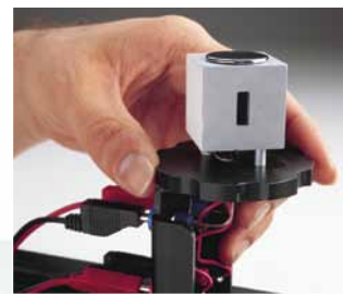
The surface of the cube is scanned with two different Light Sensors (visible and infrared).
