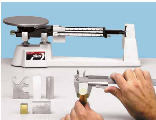
The mass and volume are measured to determine the dependence of the buoyant force on mass, volume and density.
