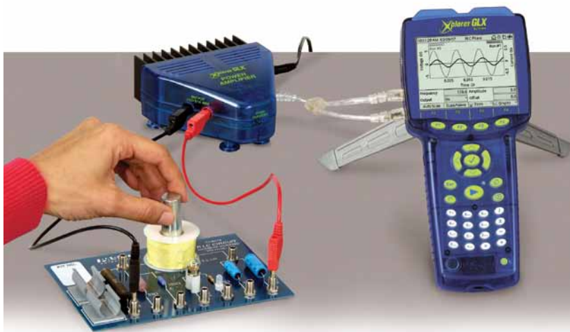
The RLC Circuit Board is powered using the Xplorer GLX to control the output of the Xplorer GLX Power Amplifier.
