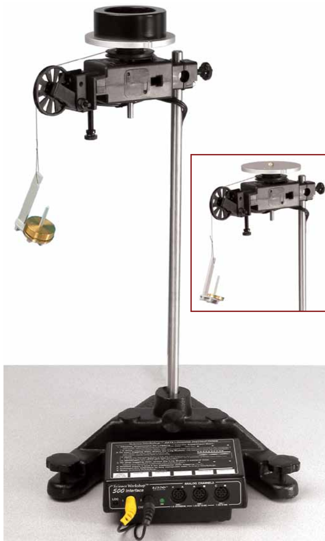
A known torque is applied to the ring and disk by the weight hanging over the pulley. The rotational inertia of the ring and disk are determined from the resulting angular acceleration. The procedure is repeated for the disk alone.
