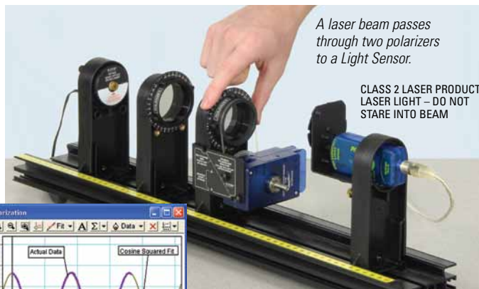
As the polarizer is rotated, the intensity of the light varies as the square of the cosine of the angle between the two polarizers.
