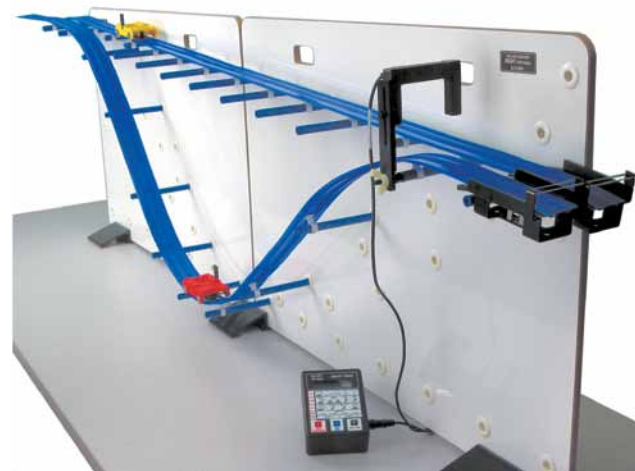
Conservation of energy shows that the final speeds of these two cars are the same even though the red car takes much less time than the yellow car to reach the end of the track.
